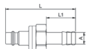
Hose Barb w/Recoil Elimin. Plug
